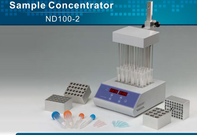
ND100-2 Sample Concentrator is with microprocessor controlled and PID fuzzy controlled technique. Instead of traditional water bath device, the heat-conducting medium is high purity aluminum. The Test tubes are held in a bolck, and blowing a large number of samples at one time.
